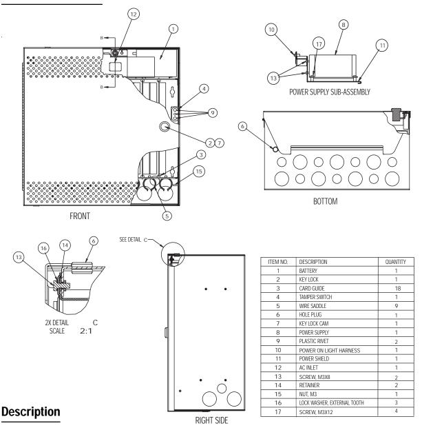
The PW-5000 system is designed for maximum efficient use of wall space through the use of a secure metal cabinet (PW5K1ENC1) that can hold up to 9 modules, a 4 amp power supply and a self-contained replaceable backup battery.
